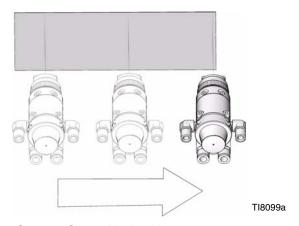
Fig. 15: Correct Spray Method
